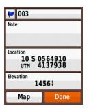
From the main menu select Mark Waypoint. The Mark Waypoint screen will appear. The waypoint will have a sequential 3 digit number assigned as its default name. and your current location and elevation will be displayed.
