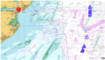
A GLONASS receiver (red dot) on England's east coast gave position fixes in the North Sea (blue triangles) BBC 9/14/2014
